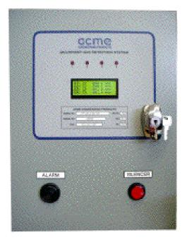
The ACME CEW4 series is a microprocessor-based up to 4 channels multigas wireless detection and control system that can be used with a wide variety of ACME toxic, combustible, refrigerant & oxygen gas sensors. The sensors can be grouped in any combination. The communication between the Control Panel and the remote Sensor-Transmitters is accomplished through a 900 MHz or 2.4 GHz wireless network.
