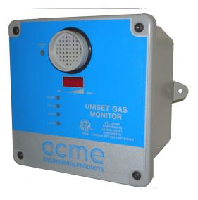
The Acme UniSet, with its microprocessor-based system, features a high quality stand-alone controller providing all the necessary hardware for the continuous monitoring of a variety of toxic and combustible gases. This unit is primarily geared towards providing alarm activated relays for simple applications such as small parking garages.
